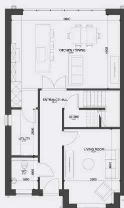
Ground Floor Plan.
